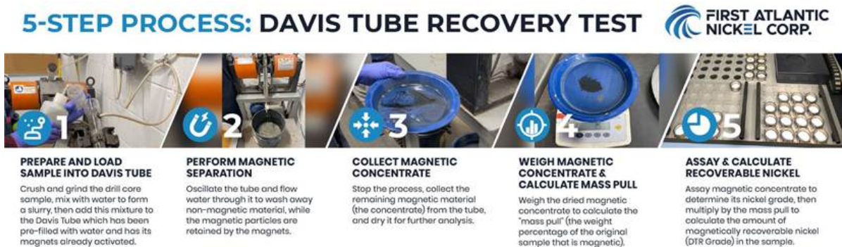
Figure 11: Davis Tube Recovery (DTR) Metallurgical Test 5 Step Process
