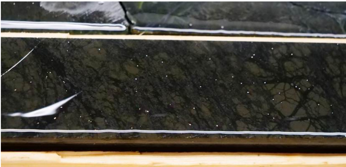
Figure 3: Example photograph of large grain awaruite ( \text{Ni}_3\text{Fe} Nickel-Iron-Cobalt Alloy) visible in drill core from the RPM Zone at the Pipestone XL Nickel Alloy Project.
