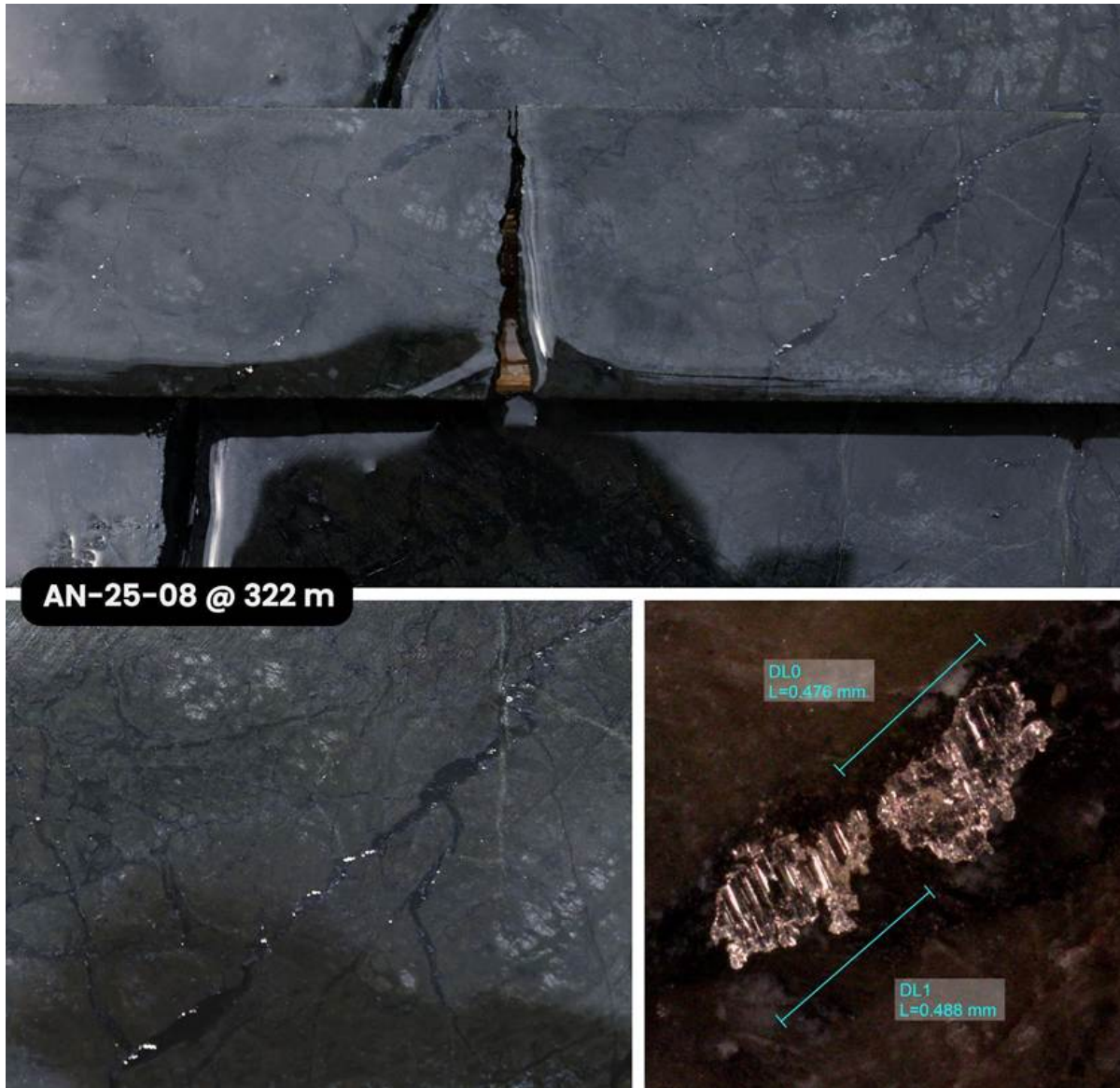
Figure 2: Drill core from hole AN-25-08 (332 m) showing unique chain formation of awaruite (nickel-iron alloy) mobilizing and concentrating along magnetite veins in serpentinized peridotite (top); photomicrographs of awaruite grains up to ~490 microns (bottom).
