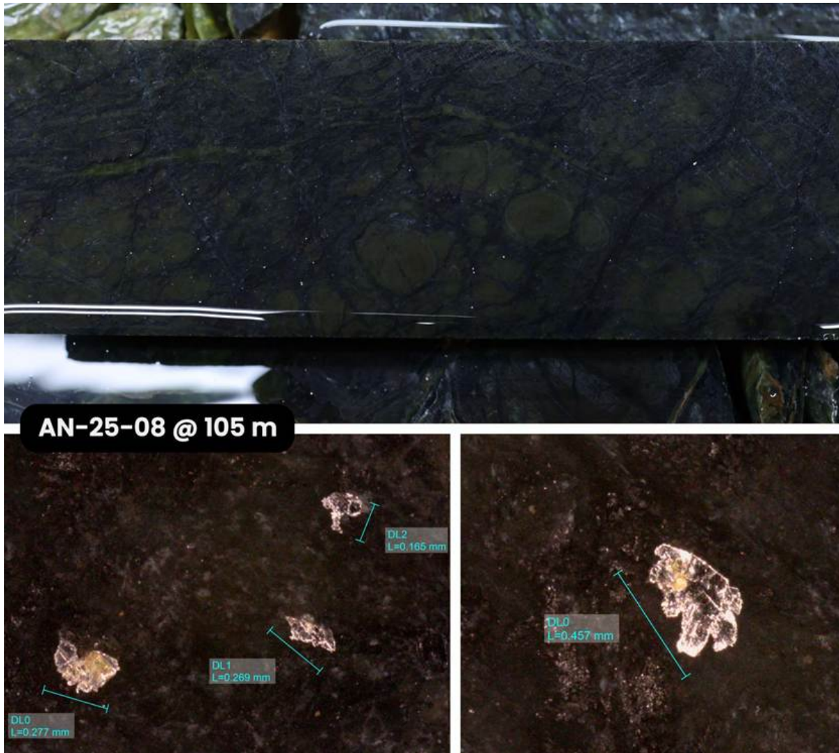
Figure 3: Drill core from hole AN-25-08 (105 m) showing disseminated awaruite (nickel-iron alloy) in serpentinized peridotite (top); photomicrographs of awaruite grains up to ~460 microns (bottom).
