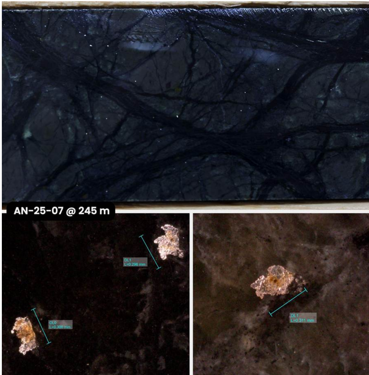
Figure 2: Drill core photograph from hole AN-25-07 at 245 meters showing disseminated awaruite nickel-alloy mineralization (top), with microscope images of awaruite grains up to 311 microns in size (bottom). Awaruite, a rare, highly magnetic, and ductile nickel-alloy can be seen disseminated within serpentinized ultramafic rocks present over significant areas on the Atlantic Nickel Project.
