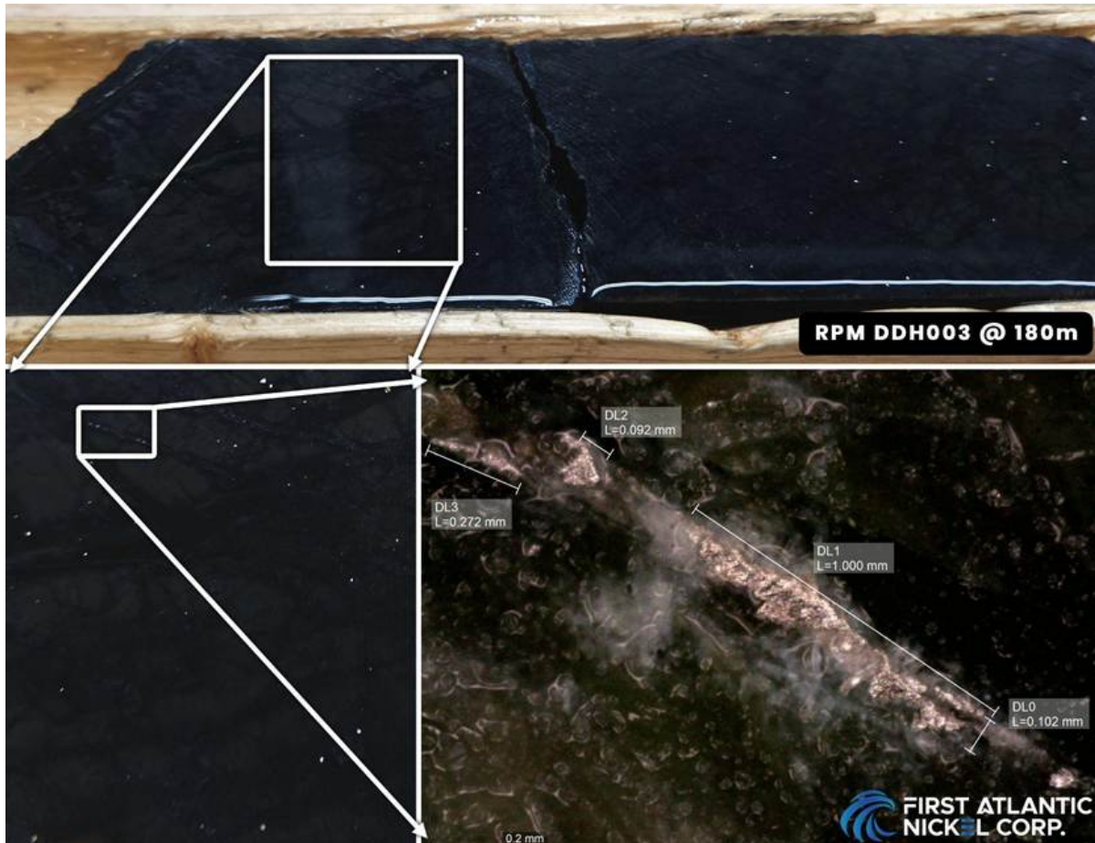
Figure 3: Core sample from drill hole RPM-DDH003 (AN-24-04) at a depth of 180 meters, featuring visible awaruite mineralization. The lower images showcase magnified views of the awaruite grains, displaying smooth and grooved surface textures. An elongated awaruite nickel-alloy grain, measuring up to 1,000 microns in size, is observed forming as a fracture filling, while average visible grain sizes range from 100 - 600 microns.
