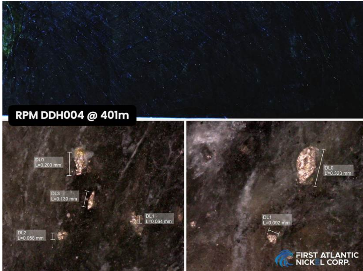
Figure 5: RPM Hole 4 Drill Core (AN-24-05) at 401 meters depth. Top image: Abundant, visibly disseminated awaruite grains (typically 50-100 microns, with some up to 323 microns). Bottom image: Awaruite grains from RPM DDH004 at 401 meters depth under a microscope, showing grains well above 10-micron size required for effective magnetic separation and recovery.
