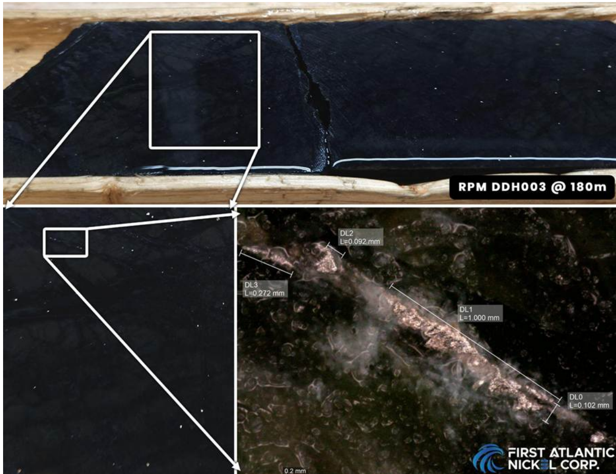
Figure 4: Core sample from drill hole RPM-DDH003 (AN-24-04) at a depth of 180 meters, featuring visible awaruite mineralization. The lower images showcase magnified views of the awaruite grains, displaying smooth and grooved surface textures. An elongated awaruite nickel-alloy grain, measuring up to 1,000 microns in size, is observed forming as a fracture filling, while average visible grain sizes range from 100 - 600 microns.
