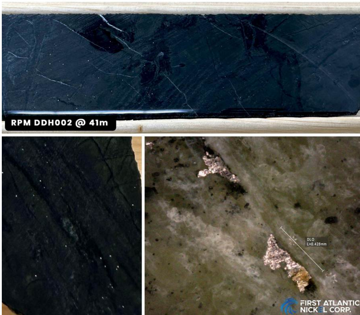
Figure 4: Core sample from RPM Drill Hole 2 (AN-24-03) at a depth of 41 meters, showing visible awaruite grains. The lower images display magnified views of these grains under a microscope, with sizes reaching up to 428 microns.
