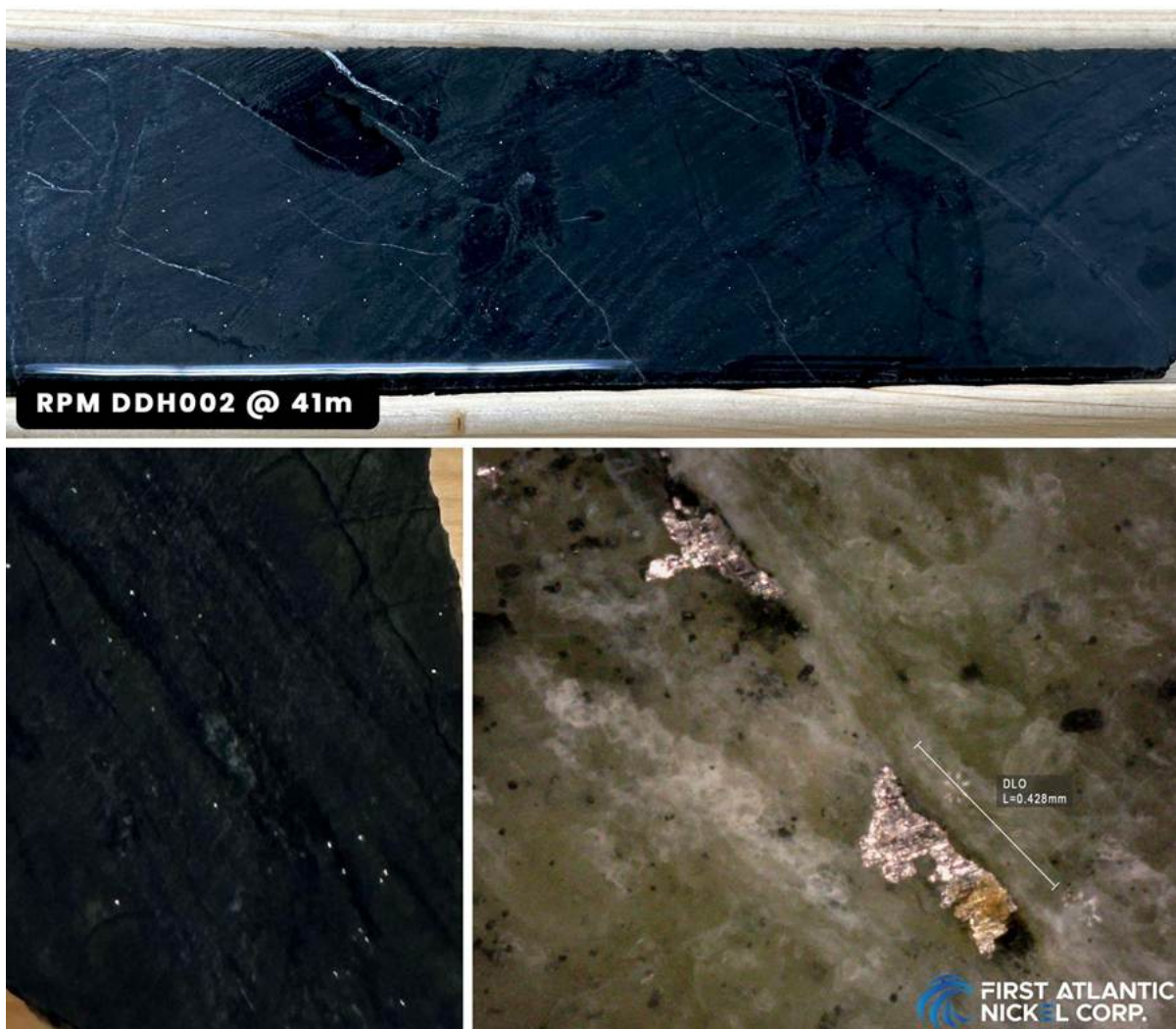
Figure 3: Core sample from RPM drill hole 2 (AN-24-03) at a depth of 41 meters, showing visible awaruite grains. The lower images display magnified views of these grains under a microscope, with sizes reaching up to 428 microns.
