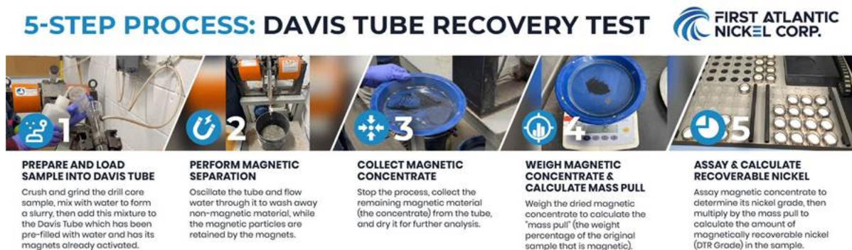
Figure 4: Davis Tube Recovery (DTR) Metallurgical Test 5 Step Process
