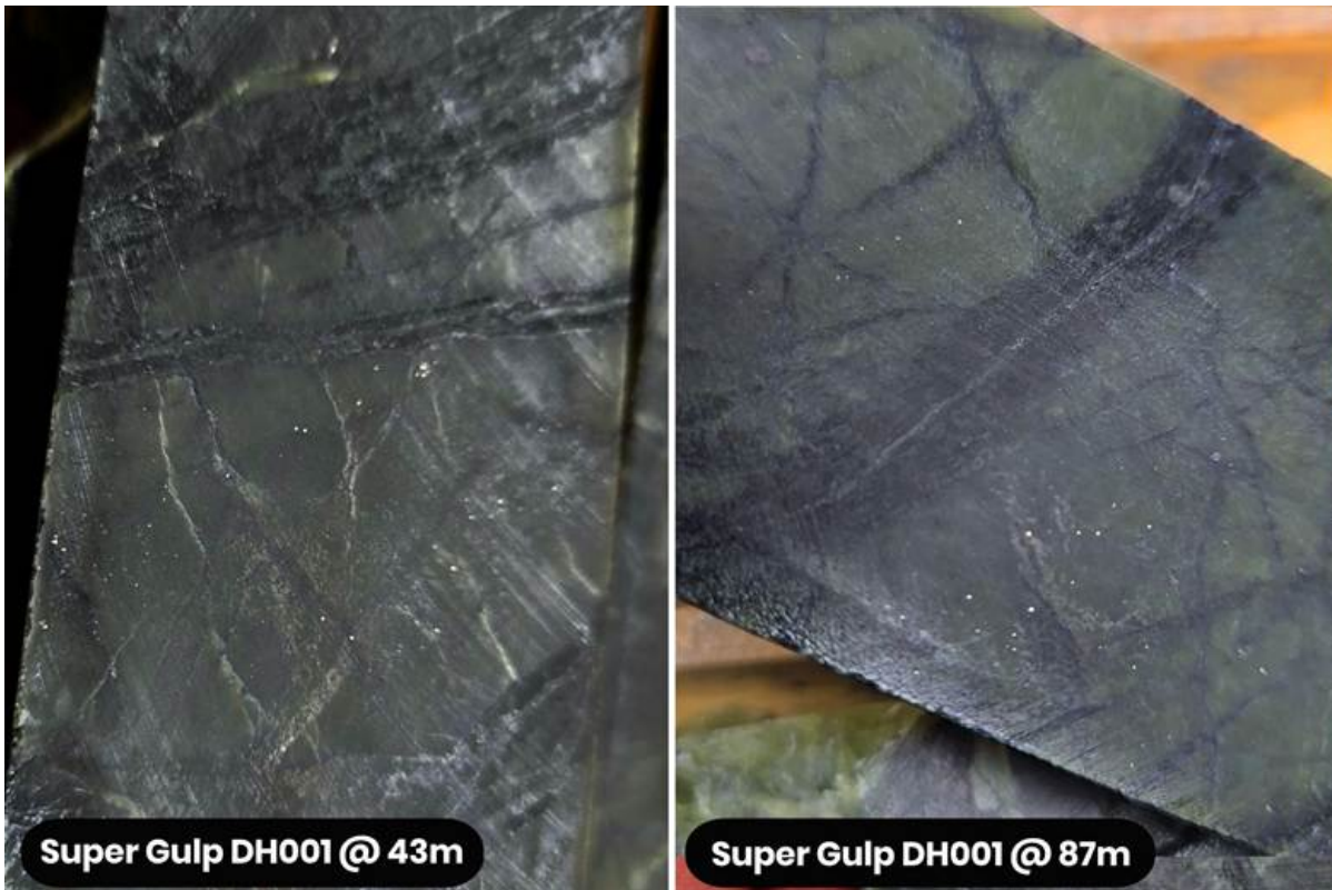
Figure 2: Super Gulp Drill Hole 1 (AN-24-01) showing disseminated sulfur-free-nickel (awaruite) in serpentinized ultramafic rock, with serpentine-magnetite fracture filling and veinlets at 43m and 87m downhole.
