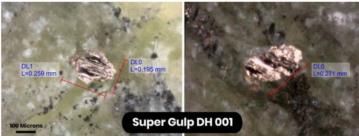
Figure 3: Microscope images of awaruite grains (~200-271 microns) in Super Gulp Drill Hole 001 (AN-24-01).
