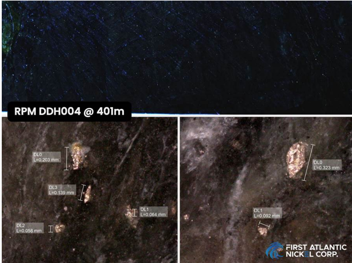
Figure 3: Drill core RPM DDH004 at 401 meters depth. Top image: Abundant, visibly disseminated awaruite grains (typically 50-100 microns, with some up to 323 microns). Bottom image: Awaruite grains from RPM DDH004 at 401 meters depth under a microscope, showing grains well above 10 micron size required for effective magnetic separation and recovery.
