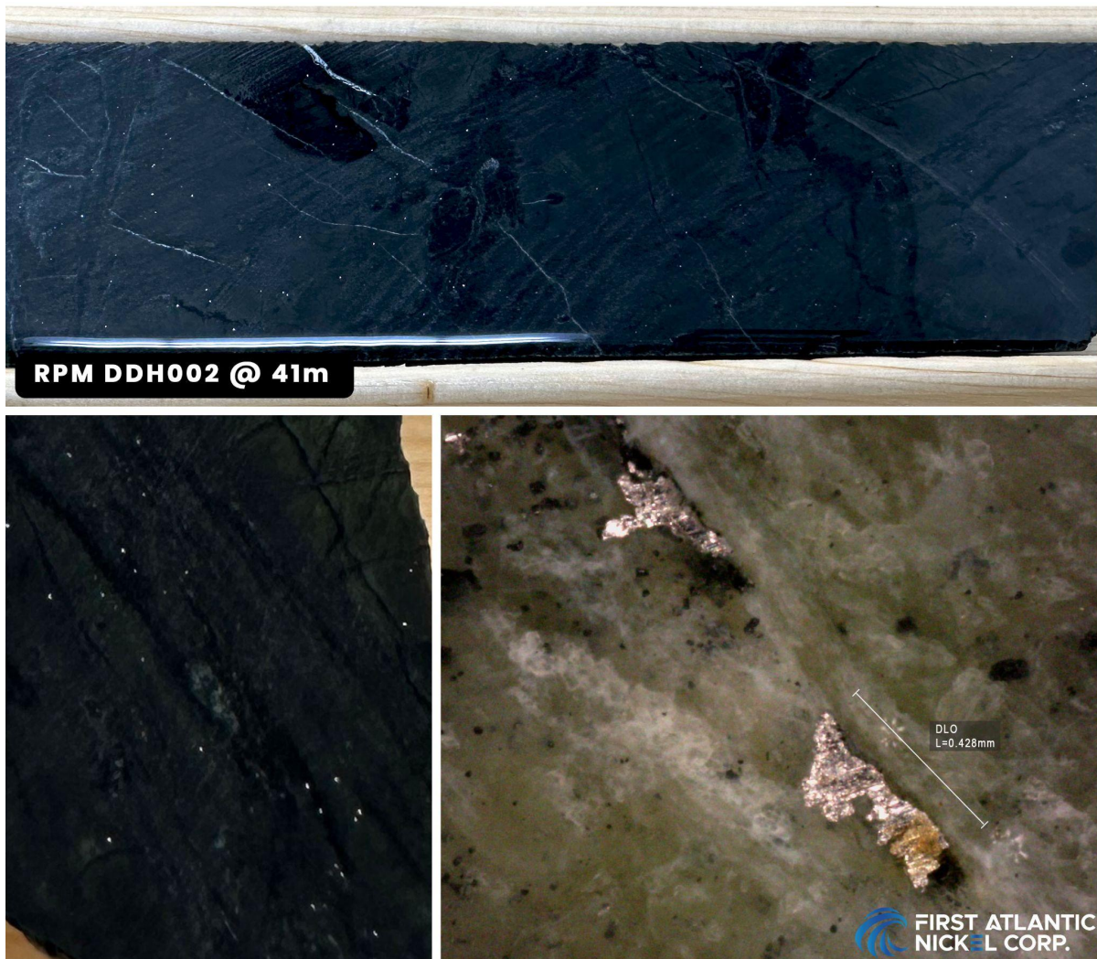
Figure 6: Core sample from drill hole RPM-DDH002 at a depth of 41 meters, showing visible grains of awaruite. The lower images present magnified views of the awaruite grains under a microscope, with sizes up to 428 microns.
