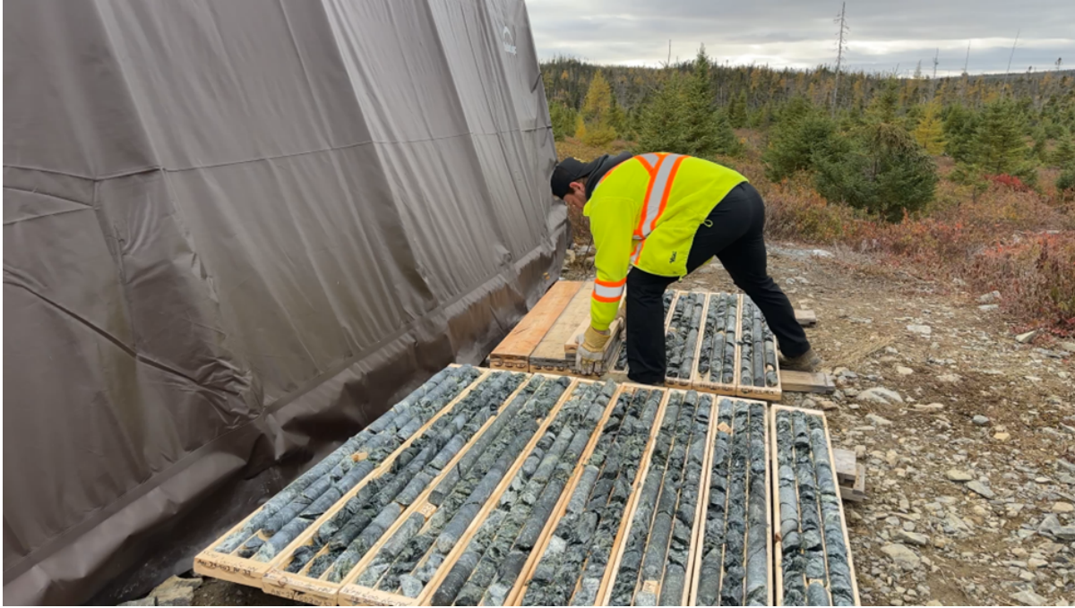
Figure 2: Phase 1 drill core being prepared for shipment from the temporary project core-logging tent.
