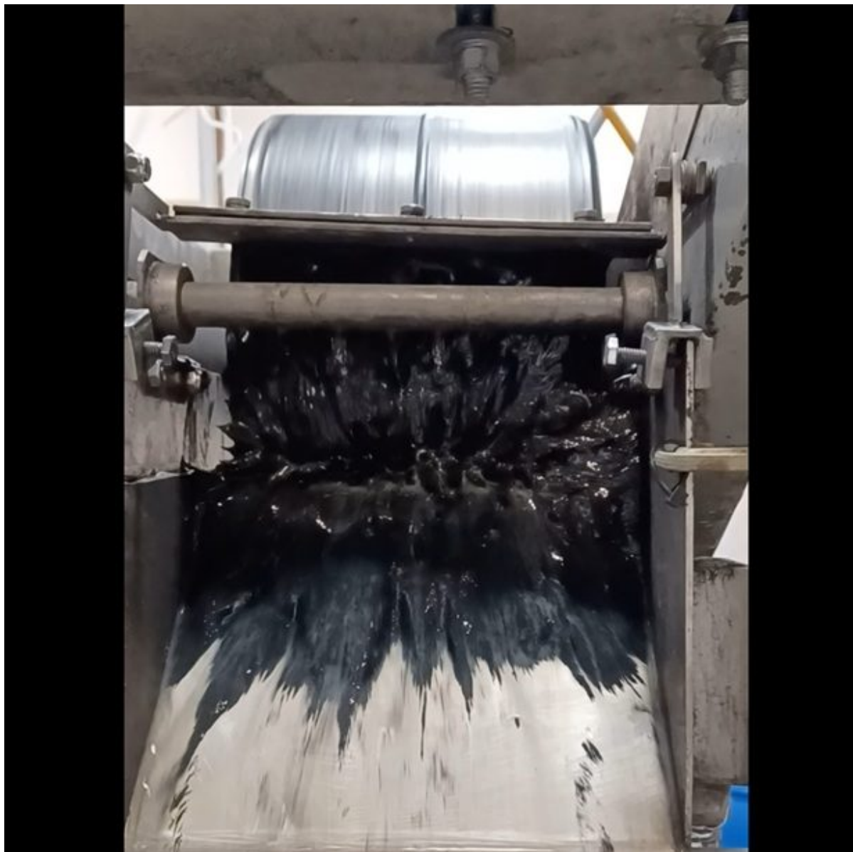
Figure 2: Image of Eriez laboratory drum separator collecting magnetic concentrate while operating at a magnetic intensity of approximately 1,000 Gauss, Low Intensity Magnetic Separation (LIMS) process.
