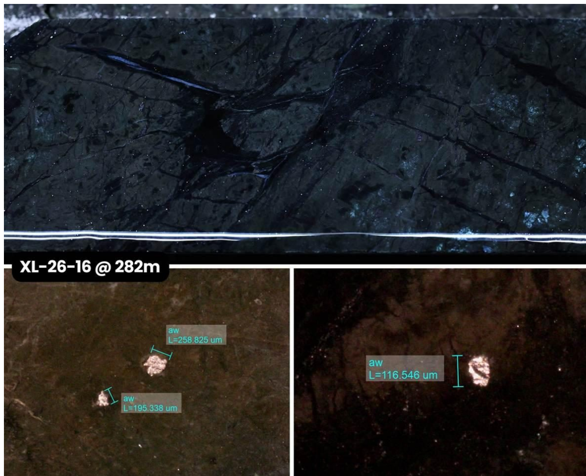
Figure 4: Visible awaruite grains measuring up to 259 microns in drill core from hole XL-26-16 at 282 meters downhole, showing the consistent awaruite visible to the naked eye that continues to the end of the hole, Alloy Max Zone, Pipestone XL Project.
