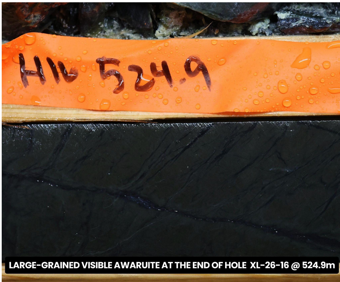
Figure 1: Visible awaruite nickel-cobalt (Ni-Fe-Co) alloy grains disseminated and concentrated along magnetite veins, within serpentinized peridotite (ultramafic) rock at the end of drill hole XL-26-16 - 525 metre total depth, Alloy Max Zone, Pipestone XL Project.
