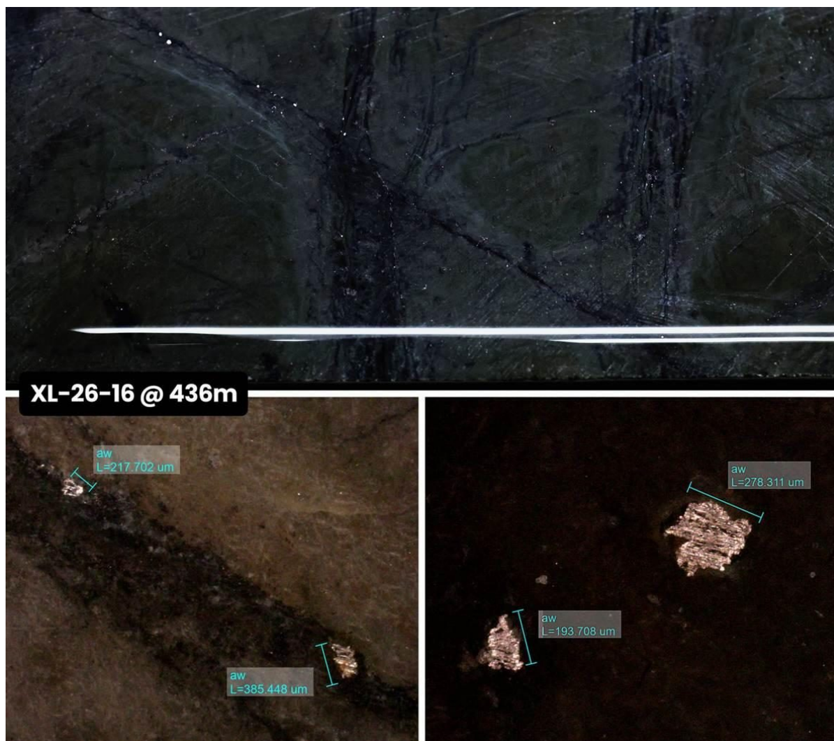
Figure 5: Visible awaruite grains measuring up to 385 microns in drill core from hole XL-26-16 at 436 meters downhole, approaching the deepest interval drilled to date at Pipestone XL. The hole ended in mineralization at 525 meters downhole.
