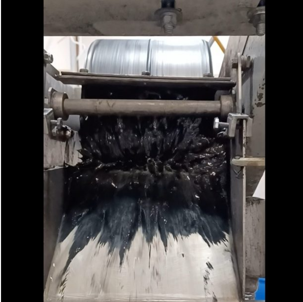
Figure 4: Image of Eriez laboratory drum separator collecting magnetic concentrate while operating at a magnetic intensity of approximately 1,000 Gauss, Low Intensity Magnetic Separation (LIMS) process.
