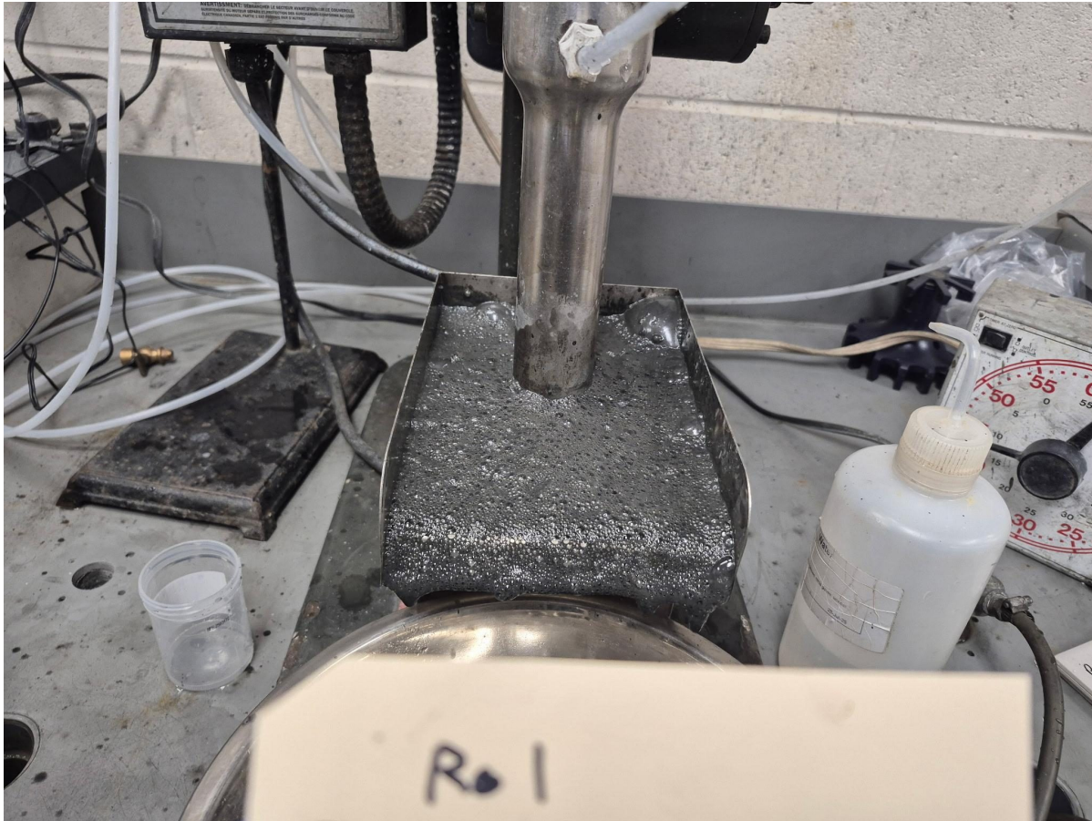
Figure 2: Preliminary metallurgical test of composite material from RPM zone at Pipestone XL project, picture showing the rougher flotation stage. The metallic surface visible on-top of liquid within a bench scale flotation cell is awaruite particles attaching to the surface of bubbles and floating to the top to be collected and cleaned in a multi-stage process isolating and concentrating the awaruite nickel-iron-cobalt alloy metal.
