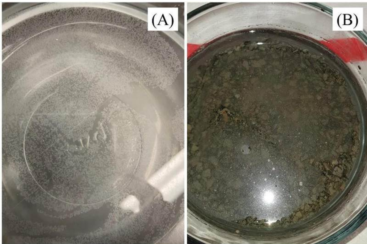
Figure 03: Carbon Sequestration Experiment from First Atlantic’s Newly Acquired Ophiolite-X Property (Blow Me Down Massif); Photographs of white films on calcium hydroxide rich waters after the 4 hours, ultra-basic carbon sequestration experiments. (A) Without the addition of crushed peridotite and (B) with the addition of crushed peridotite. [20]
